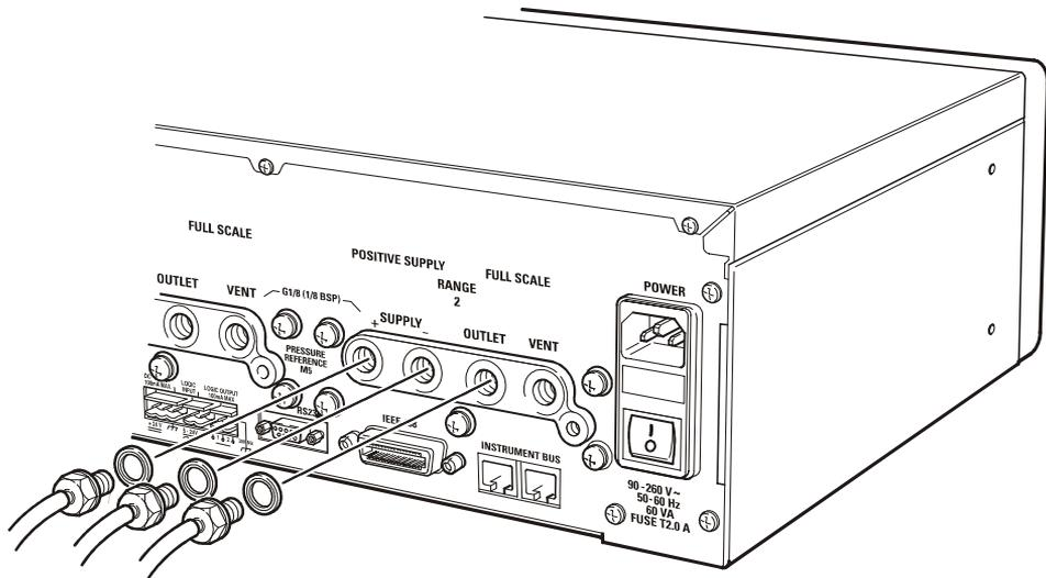
Figure 2-1, Pneumatic Connections
