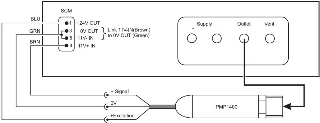
Figure 2-16, 3-wire, Amplified Voltage, Pressure Transducer Test Set-up
