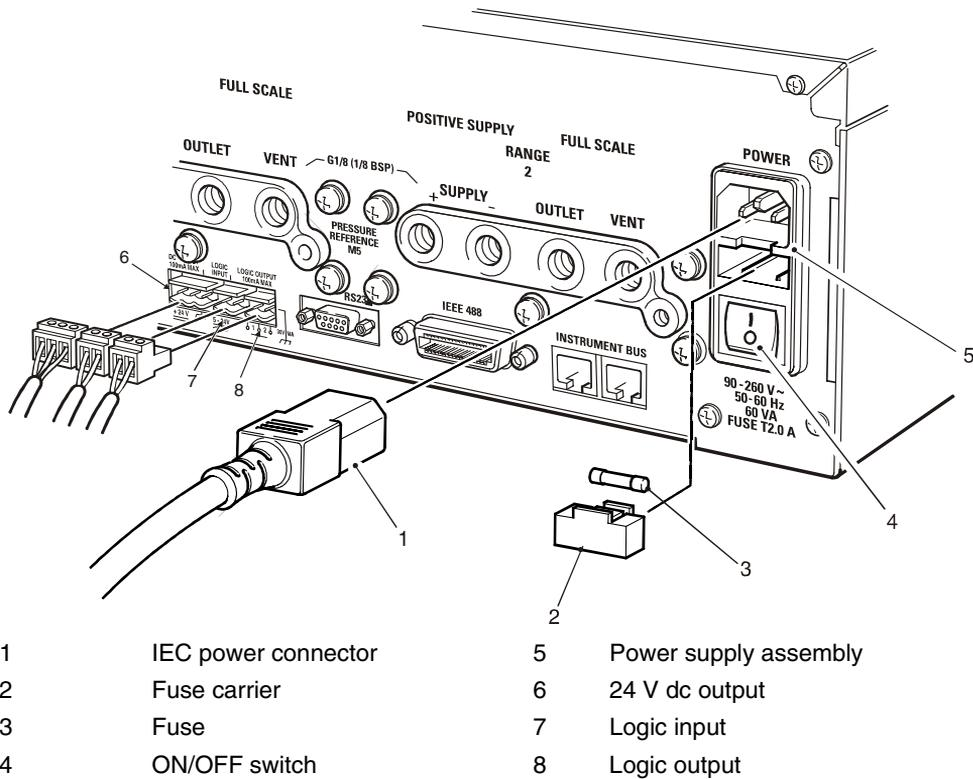
Figure 2-6 Electrical connections
