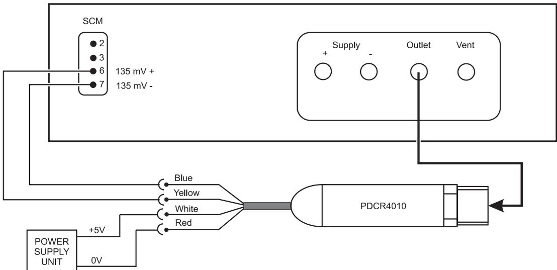
Figure 2-20, Millivolt Output Pressure Transducer Test Set-up
