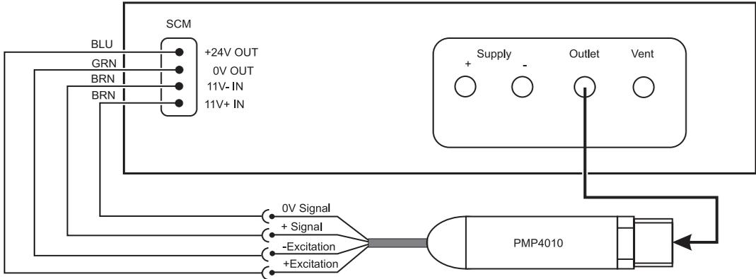
Figure 2-17, 4-wire, Amplified Voltage, Pressure Transducer Test Set-up
