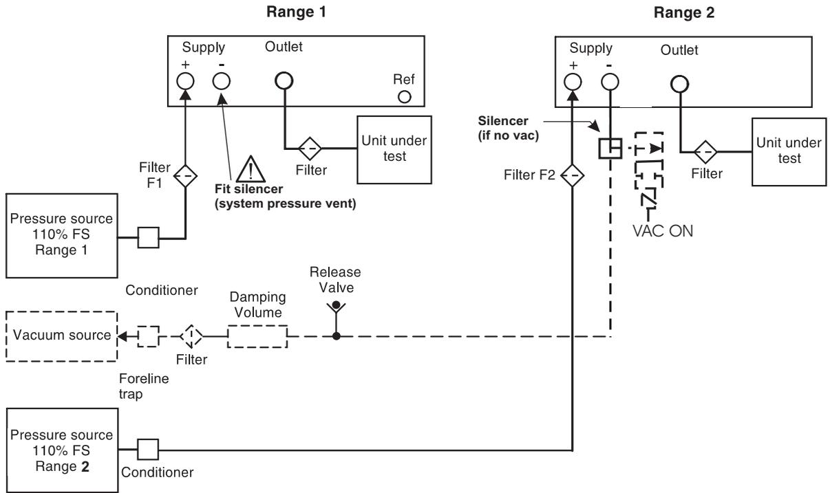
**Figure 2-4, Pneumatic Connections above 70 bar (1000 psi)**
