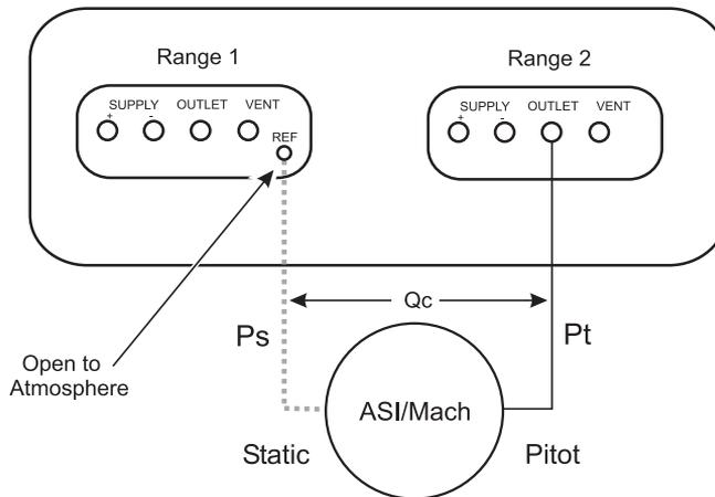
Figure 2-12, Check Airspeed Indicator or MACH meter
