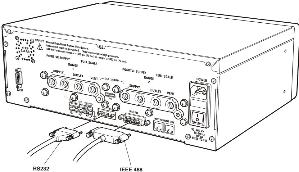
Figure 2-7, RS232 and IEEE 488 Connections
