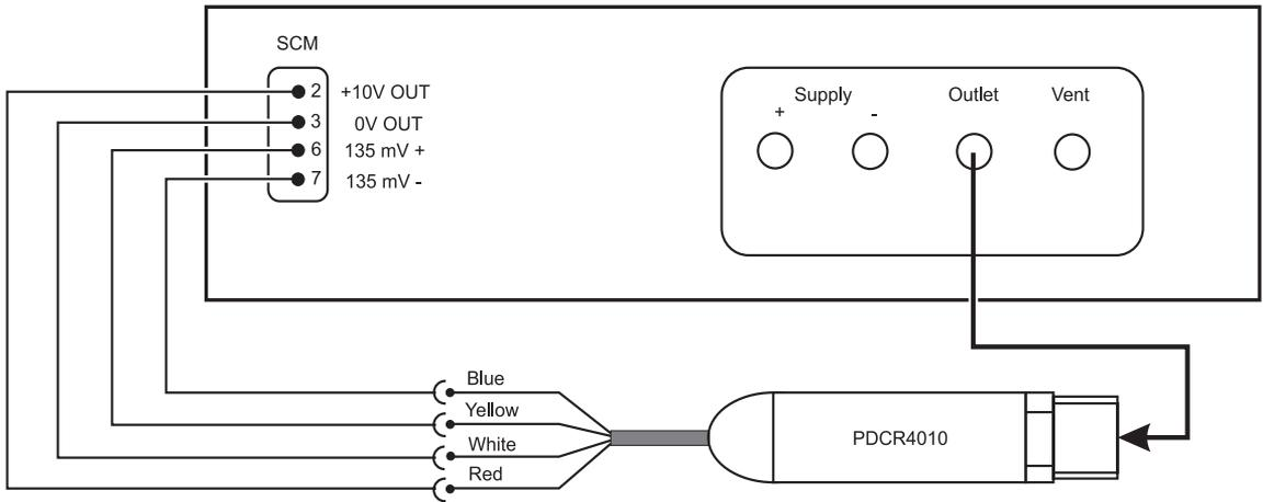
Figure 2-19, Millivolt Output Pressure Transducer Test Set-up (Compensated)
