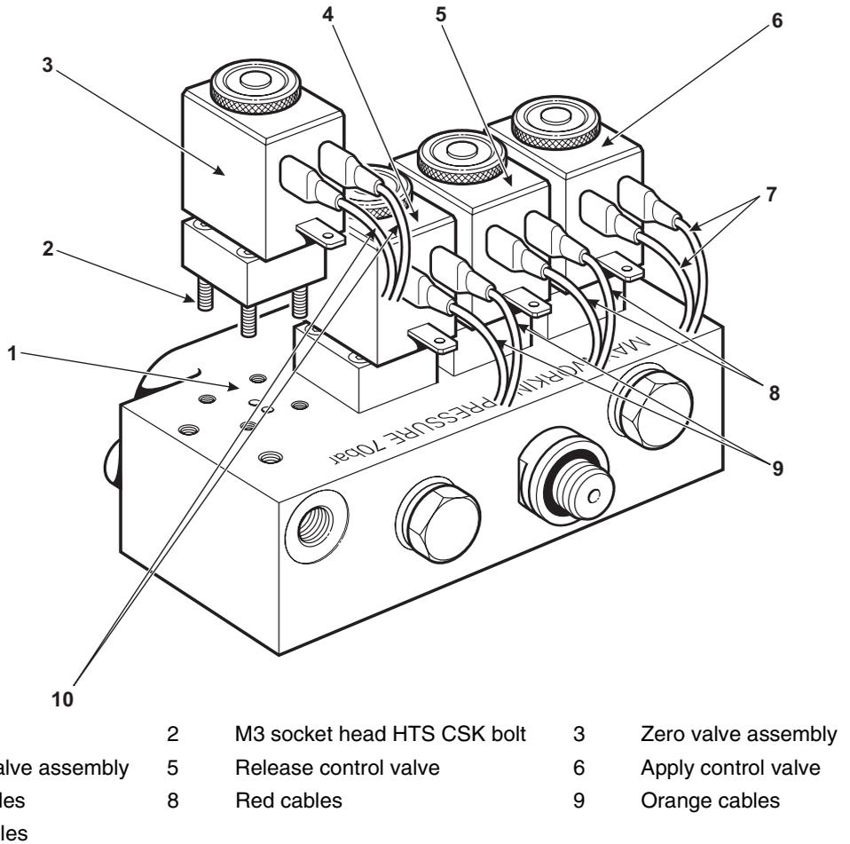
Figure 4-3, 0-70 bar (0-1000 psi) Manifold Assembly
