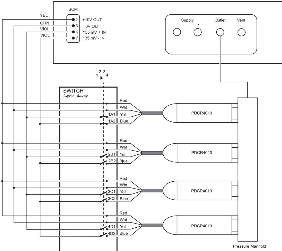
**Figure 2-21, Multiple Millivolt Output Pressure Transducer Test Set-up**
