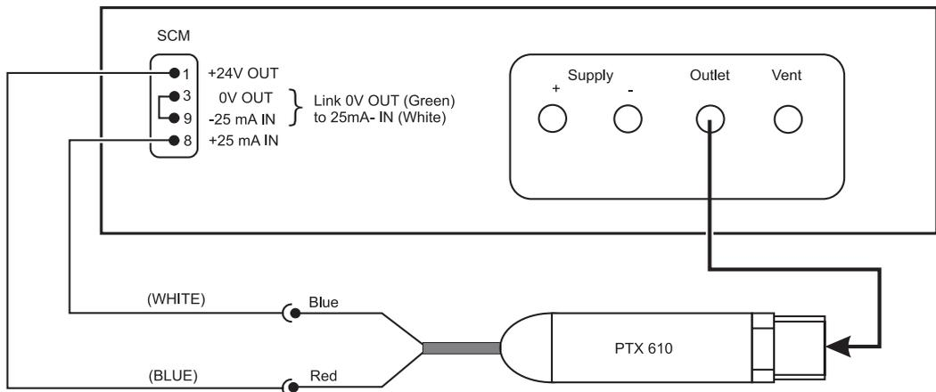
Figure 2-14, Single Pressure Transmitter Test Set-up
